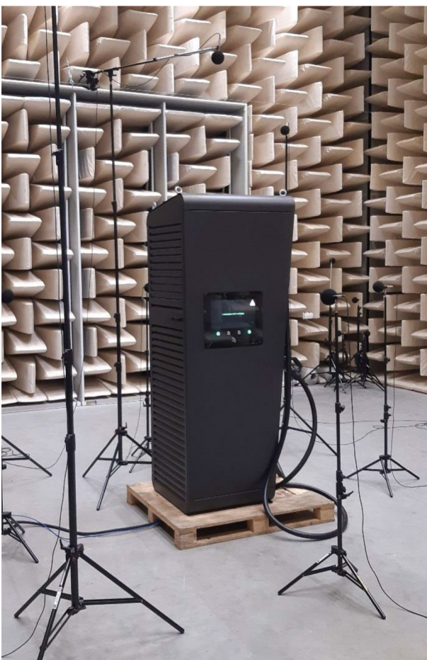
Figure 2.1 Setup Acoustic Measurement TÜV
