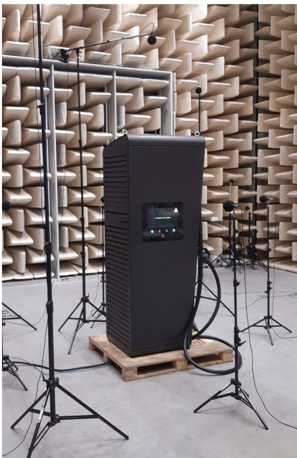
Figure 2.1 Setup Acoustic Measurement TÜV
